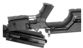
CAUTION: Selector lever should be on SAFE before closing Upper Receiver. Engage receiver pivot pin.
