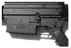
2.) Open bolt and check chamber. Make sure it is clear.
