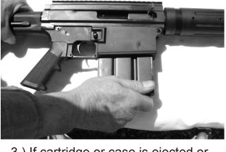
3.) If cartridge or case is ejected or chamber is clear, RELEASE charging handle to feed a new round.
